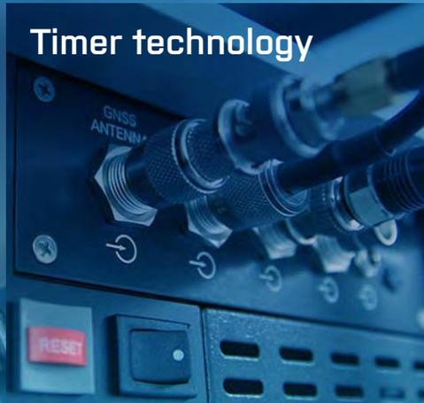
Top-quality receivers of GNSS (Global Navigation Satellite System) signals, designed for time and frequency transmission. They are used especially in metrological laboratories for comparing time and frequency standards. However, they also find their use in all applications in which it is necessary to maintain a very precise unified time over large areas, e.g., in telecommunications.
